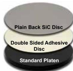
Double sided adhesive discs are adhered to a standard platen and used to secure plain back silicon carbide abrasive discs. Each provides 25-75 disc pulls depending on grit size, cycle time and force.
