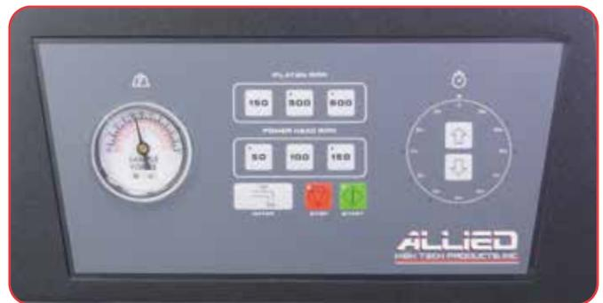
An intuitive user interface with user-friendly touchpad controls makes the E-Prep 4™ system easy to use and program. The microprocessor based system allows platen speed, sample rotation speed, cycle time and water to be controlled.
